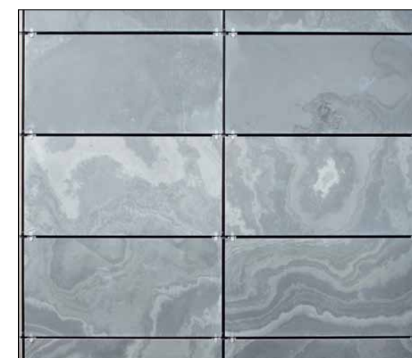
Symmetrical cladding 600 x 300 mm, laid horizontally, fastened to the aluminium substructure with stainless steel mounting clips HE130
