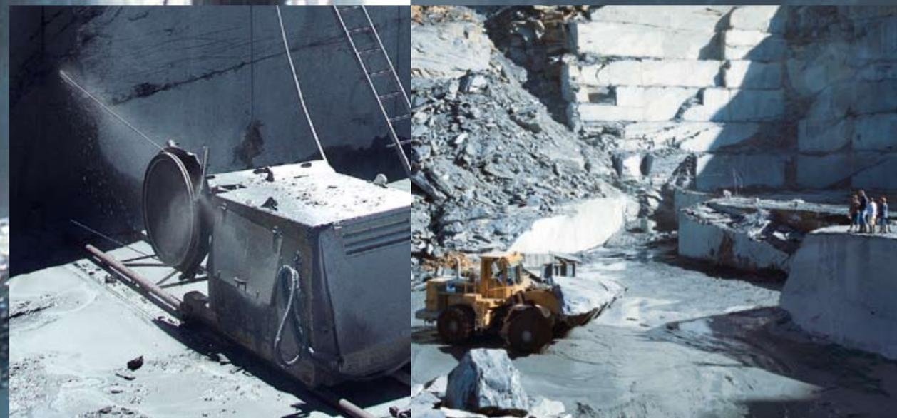
Special wire saws divide the gigantic slate blocks into even square stone blocks.
