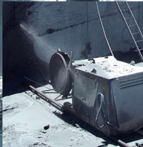
Special wire saws divide the gigantic slate blocks into even square stone blocks.
